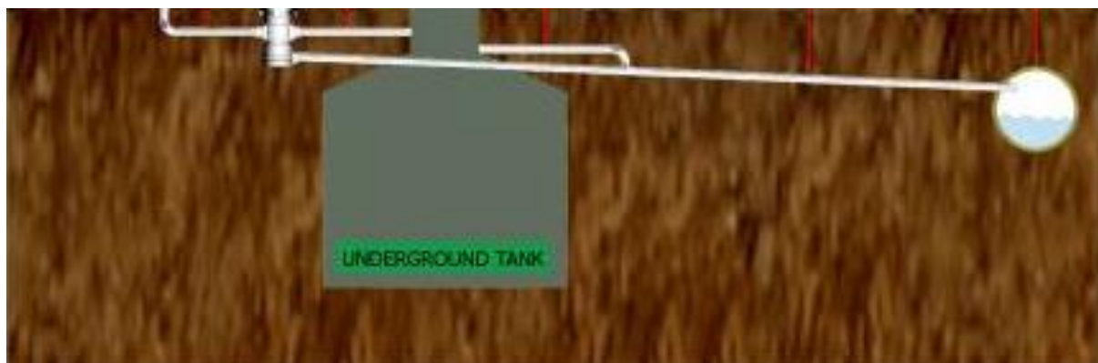
Figure 3: An in-ground first flush diverter and tank connection (source: Raindog)
