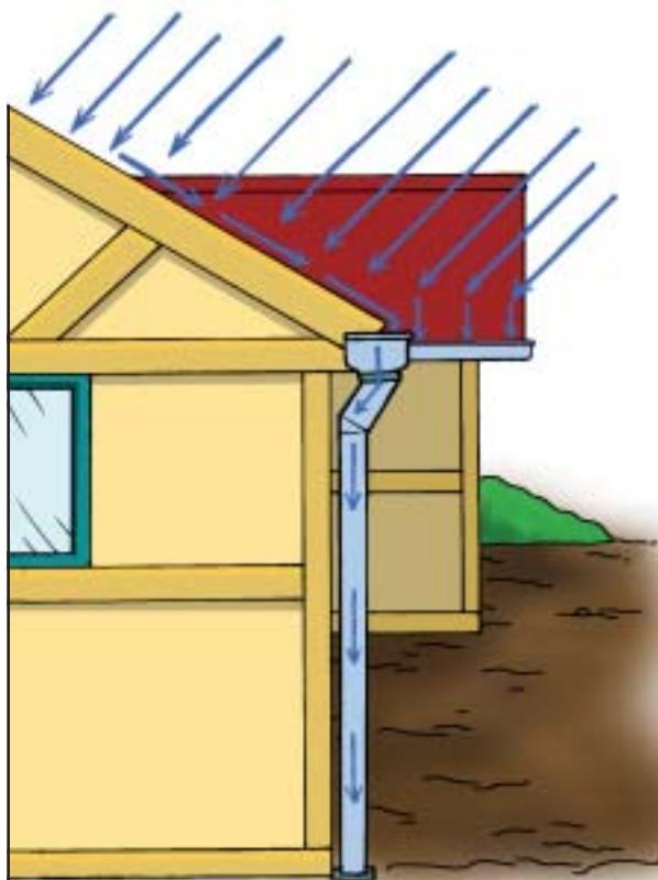
Connecting downpipes to the stormwater or onsite detention system has a number of benefits:
