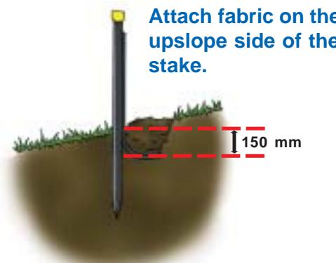
**b) Dig a trench along the fence line before temporary site fencing is installed.**
