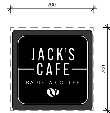
80mm DEEP INTERNALLY ILLUMINATED LIGHTBOX WITH DIGITAL PRINT TO FACE AND BLACK ACM TO EDGES ALLOW FOR POWER READY FOR FITOFF
